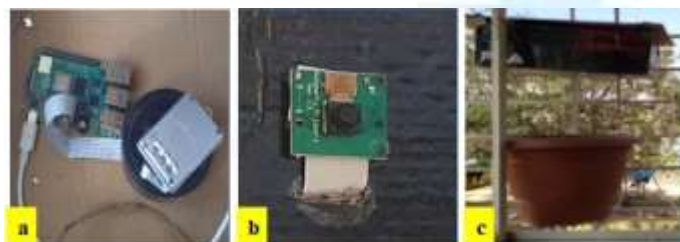
Fig. 3. Onsite model of the system (a). Raspberry Pi (b). Pi camera (c). Image collection of plant.
